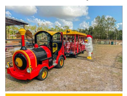
Open cabin with front & back window. Coaches are completely galvanized with powder coated frame. ADA Access Options. Can have up to 3 coaches.
