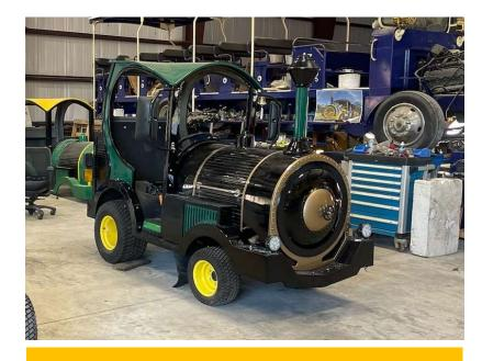
Open cabin with front & back window. Coaches are completely galvanized with powder coated frame. ADA Access Options.
